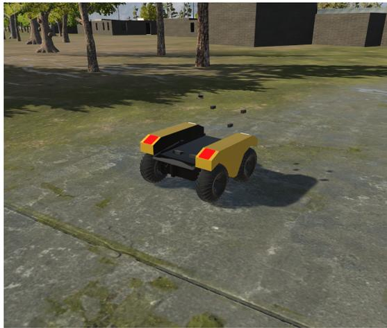
Figure 3.3: Simulated environment with Clearpath warthog running ROS equipped with an array of virtual sensors.
